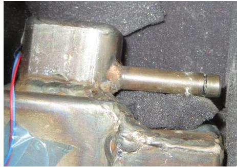
Fig. 4. CO 2 container for activating supercooled sodium acetate water mixture by cooling.
