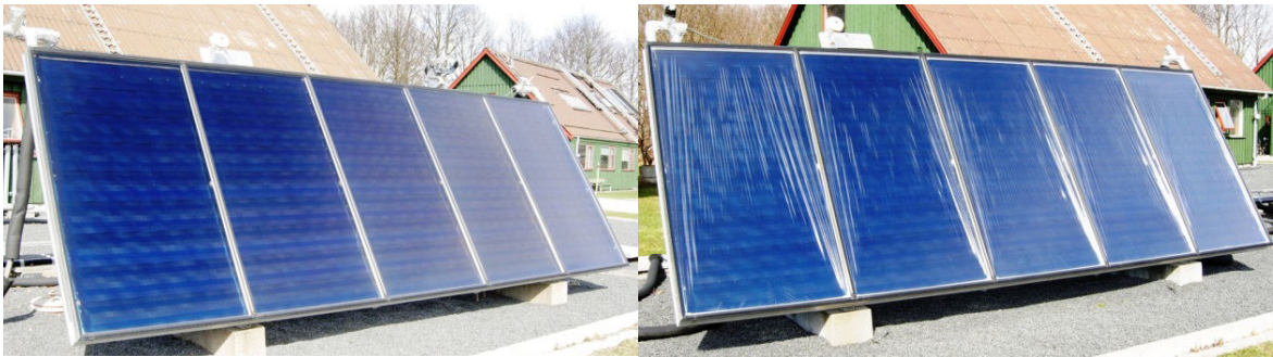
Fig. 1: Solar collector HT-A 35-10 (left) and HT-SA 35-10 (right) at the Department of Civil Engineering at the Technical University of Denmark.
