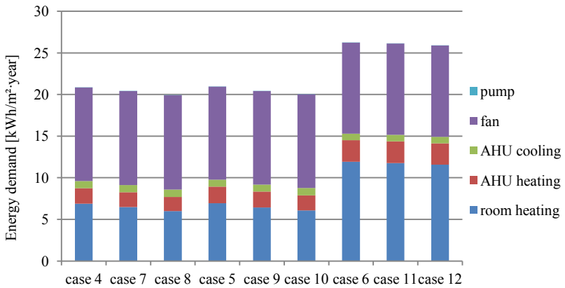
Fig. 6 Energy demand for different occupancy profiles and DPV fan power at indoor temperature of 29 °C
