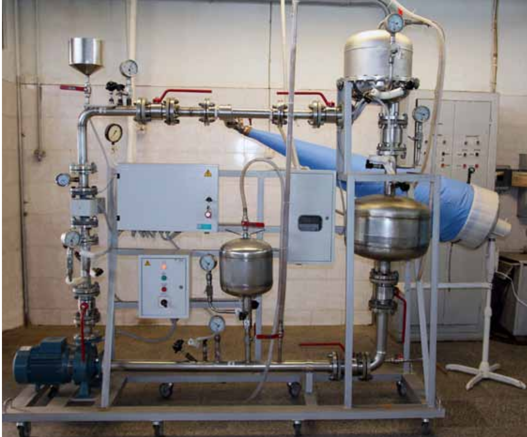
Fig. 1. General appearance of the prototype. Key elements: electric motor, centrifugal pump, suction pipeline, delivery pipeline, wind accelerator, reactor, separation tank, intermediate tank, standby tank, filling device.
