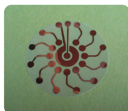
Figure 2. Gold electrodes fabricated on a PC membrane using E-beam evaporation.
