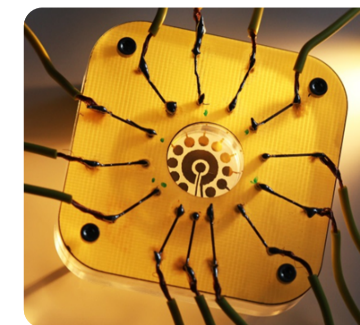
Figure 8. Device for testing membrane electrodes. The membrane holder was designed in two versions, one for bonding and one for clamping. Both were fitted with a custom PCB board for connection to a potentiostat.
