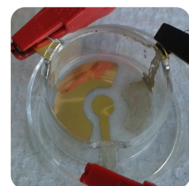
Figure 1. Membrane electrodes fabricated on a cell culture insert using sputtering. The electrodes have been fabricated in gold and silver respectively.
