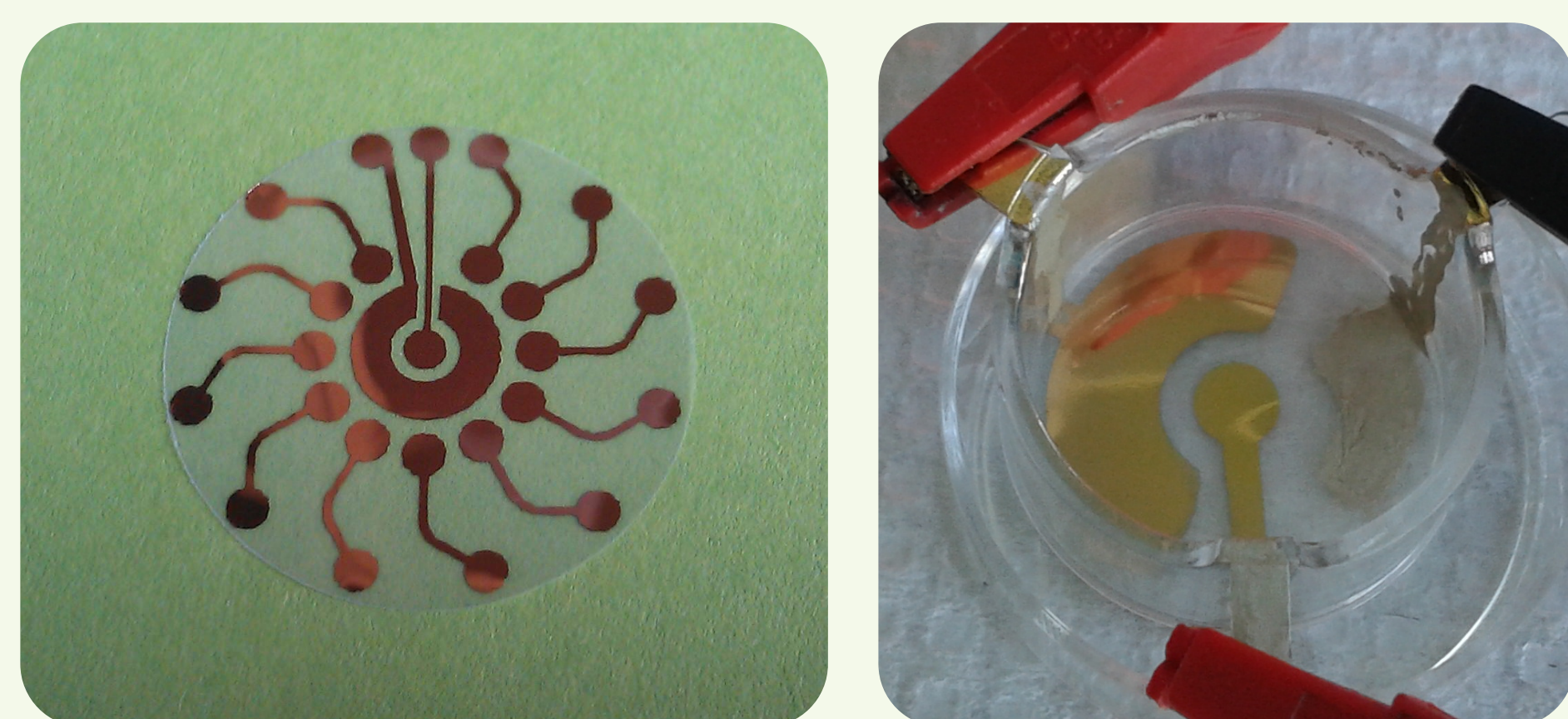
Figure 1 Membrane electrodes fabricated on two different types of membranes. Left: Gold electrodes on a flat polycarbonate membrane using E-beam evaporation. Right: Gold and silver electrodes fabricated on a cell culture insert using sputtering.
