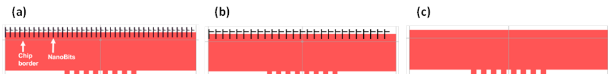
Figure 15 Tanner EDA layout editor L-Edit® snapshots of different membrane/template types. (a) Membrane with NanoBits at the edge; gray line extending across the membrane indicates the chip front-border; (b) membrane with hybrid structures; (c) a template (a long longer membrane without any patterns).
