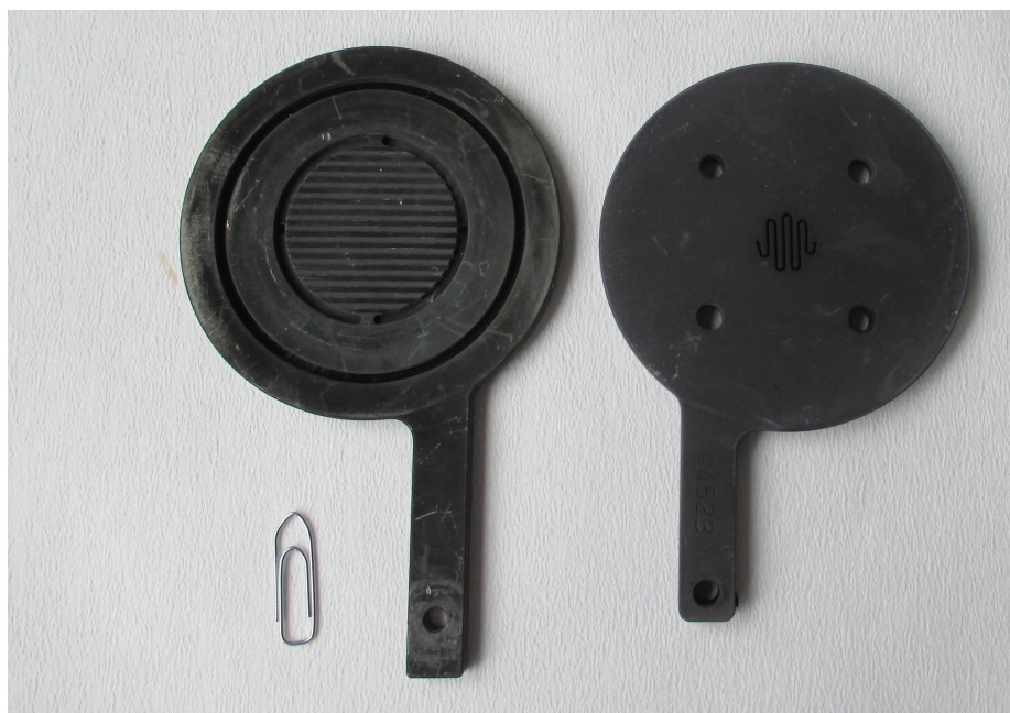
Figure 6.5: Two types of tantalum coated stainless steel flow plates. The left is of type 1 and the right is of type 3.
