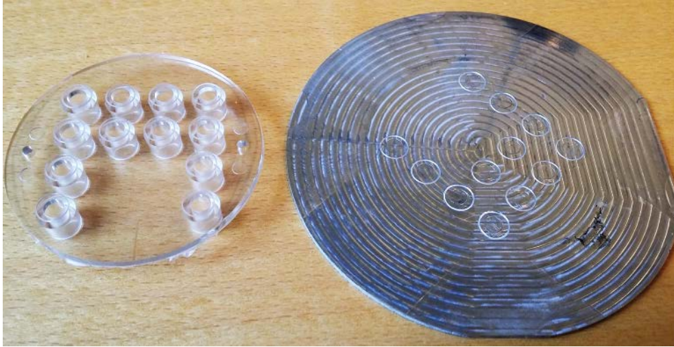
Figure A-17. Chip with 12 integrated Luer-lock connectors and mold inlay. Each connector were integrated with energy directors at the bottom side for welding.
