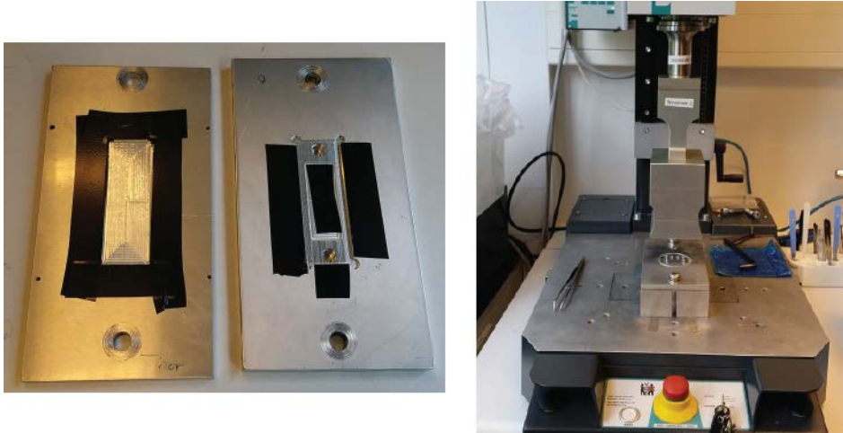
Figure A-18: Aluminum holders for bonding of the microfluidic chamber (left) and the Luer-Lock connectors to the assembly (right). To the right is the Telsonic Ultrasonics UPS-3000 welder.
