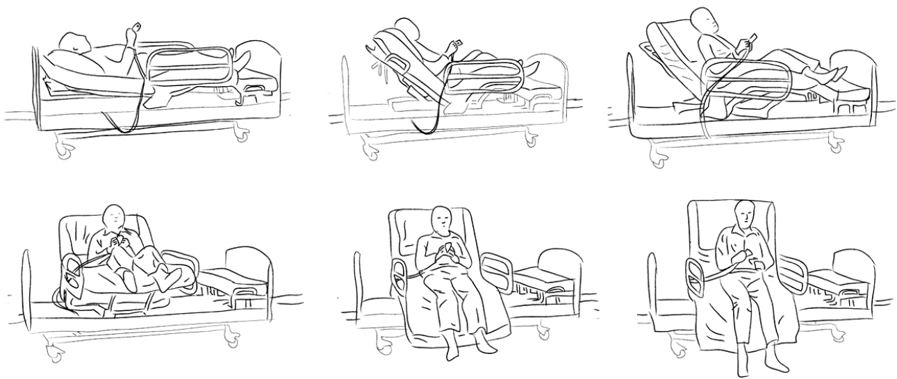
Figure 1. The rotation process of the RotoFlex bed.
