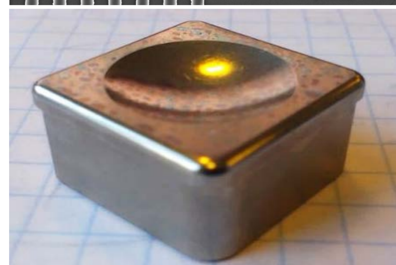
Fig. 3: Fabricated tool insert for use in this experiment.
