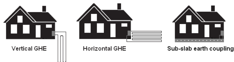
Figure 1. Ground-coupled (closed-loop) systems
