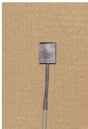
Surface temperature sensor with insulation
