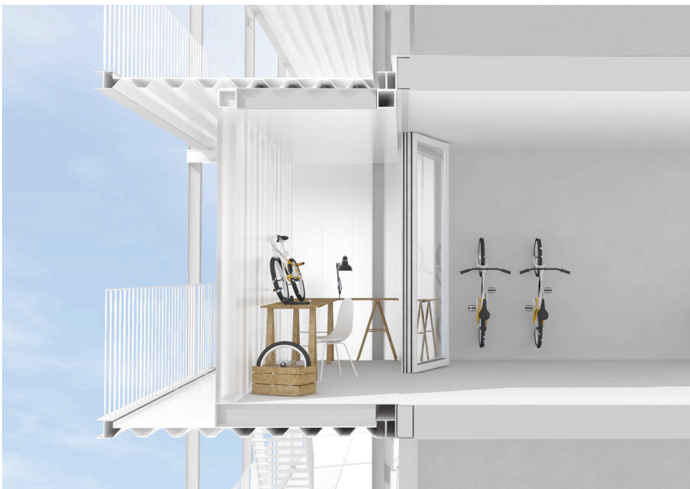
Figure 5-40 Section of deep façade with enclosed space for a live/work unit or bike storage. Design and drawing by architect Gustav Düsing.
