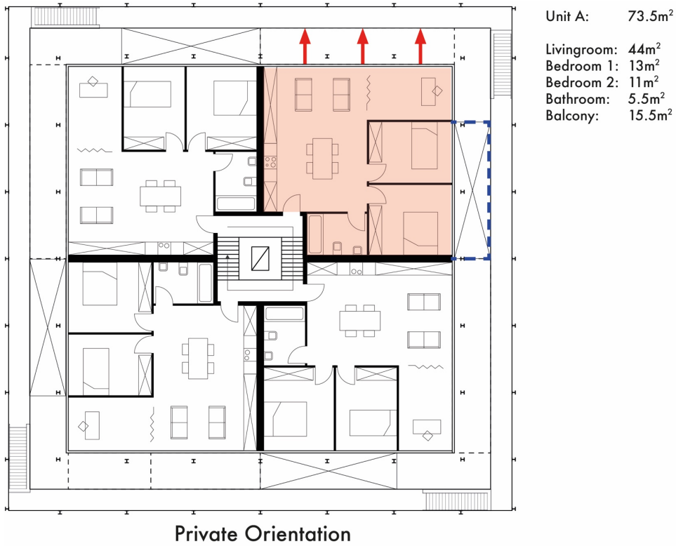
Figure 5-34 Unit A, showing the private orientation. The blue dotted line shows the cut-out for privacy next to the bedroom, which also lets light to the flat below and the red arrows show the semi-public outdoor space. Design and drawing by architect Gustav Düsing.
