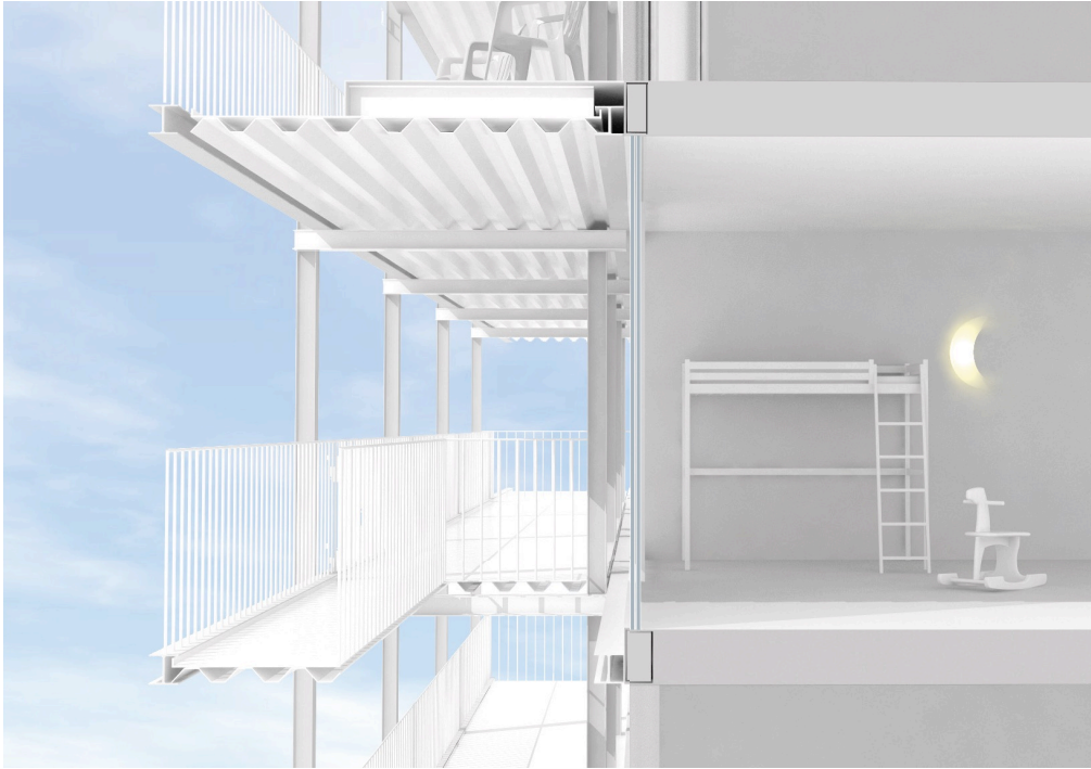
Figure 5-41 Section of deep façade showing the cut-out next to bedroom. Design and drawing by architect Gustav Düsing.
