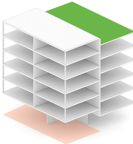
Figure 5-23 The open shelf system with cross-oriented loadbearing walls for risers allow for a differentiated space on the ground floor and roof level, to accommodate social programmes and a roof garden. Also, the split-level open shelf system on the ground floor makes it possible for half of the ground floor to be half a storey taller, indicating a change in programme and use. Drawings and design by architect Gustav Düsing.
