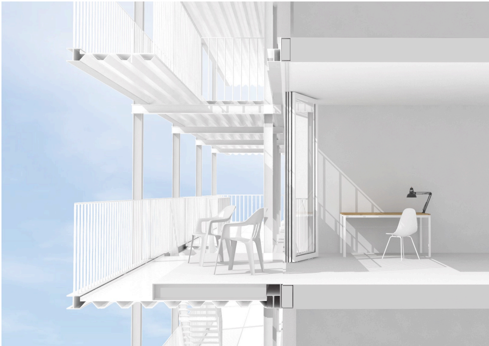
Figure 5-39 Section of deep façade with semi-private outdoor space. Design and drawing by architect Gustav Düsing.
