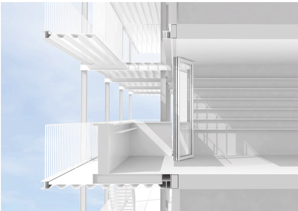
Figure 5-42 Section of deep façade with enclosed private balcony. Design and drawing by architect Gustav Düsing.
