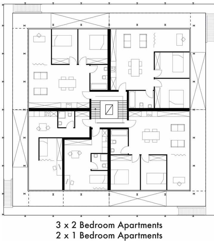
Figure 5-33 Mixed unit configuration for combination of units for between large and small households. Design and drawing by architect Gustav Düsing.
