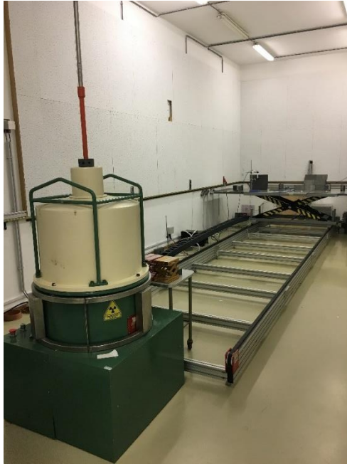
Figure 5-4: ESTEC Co-60 Radiation Cell where the steel container containing the source is shown in the foreground, with a positioning trolley shown capable of positioning DUTs between 40 cm and 815 cm. The CIS115 during testing are placed 55 cm from the source.
