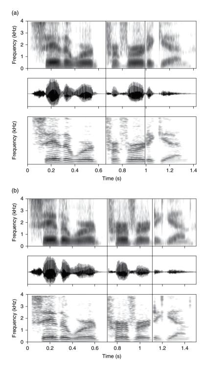
**Figure 9.1** Sound spectrograms of the words *perVERT* (a) and *PERvert* (b) in the carrier sentence *Say the word . . . again,* recorded by a male speaker of American English. Each figure consists of three display panels: (top) a broad-band spectrogram; (middle) a waveform display; and (bottom) a narrow-band spectrogram. Vertical lines indicate onset and offset of *pervert*. The figure is modeled on a figure first presented by Lehiste and Peterson (1959, p. 434).
