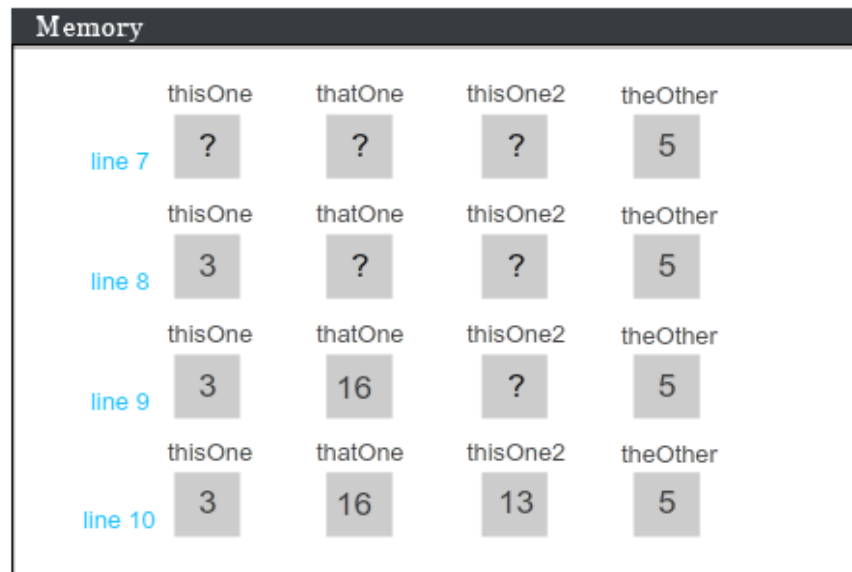
Figure 5.8 The Memory box. The line numbers ‘line 7’ to ‘line 10’ are displayed in blue. If a variable’s value is changed in the statement, the variable diagram box will be circled in red.
