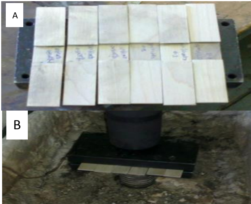
Figure 3.5: (A) six adhesive nanocomposite bonded samples on a metal bar (B) bonded wood samples pressed by the hydraulic machine inside the furnace at a constant temperature and pressure.
