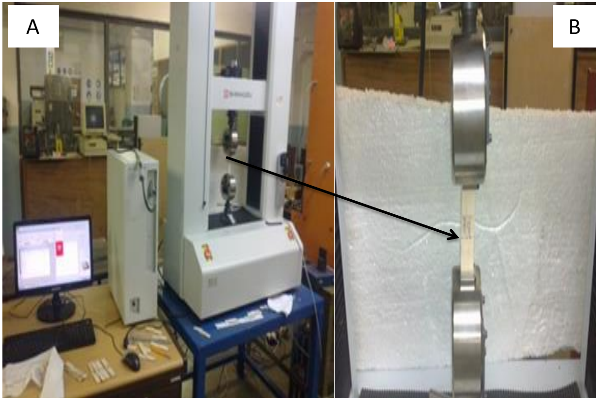
Figure 3.7: (A) Set-up of tensile testing machine with a computer system showing the readings/data values (AG-IC 20/50 KN Shimadzu) (B) Bonded wood sample clamped to the tensile test machine.
