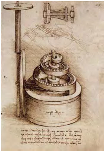
Figure 4. Codex Madrid I, 45r Technique to regulate springs
