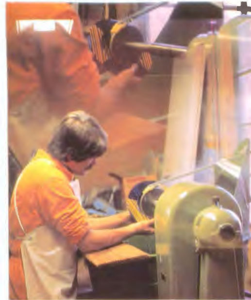
Fig. 36. Klaus Moje grinding inside curve of fused glass bowl using glass lathe and diamond cutting wheel.
