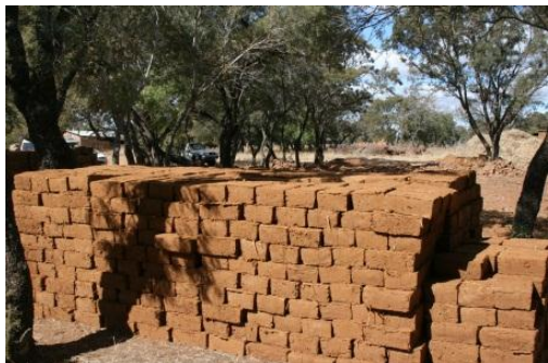
The handmade bricks that were used for the compost toilet. The bricks are made from soil and grass found in the area, and baked in the sun.
