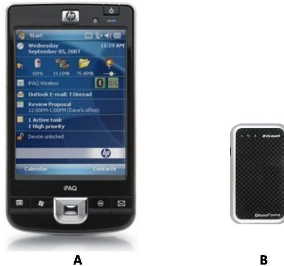
Figure 3.2 Data-collection hardware (a) HP iPAQ 211 PDA ( http://www.hp.com ), (b) Globalsat BT-368i Bluetooth GPS receiver ( http://www.usglobalsat.com/ )
