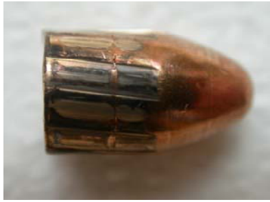
Figure 2.2 Rifling impressions on a fired bullet (Thomas, 2005:18)
