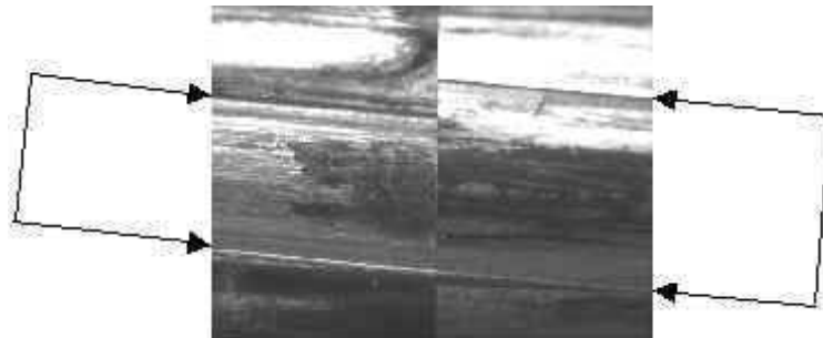
Figure 4.4 Microscopic comparison of land impressions of two fired bullets fired from different firearm barrels (Photo taken by the researcher).
