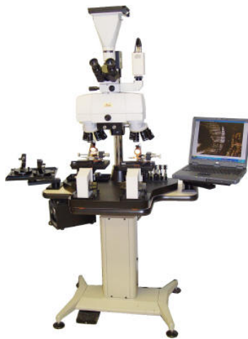
Figure 4.2 The Leica comparison microscope with a laptop for a live view of the images being examined ( www.firearmsid.com assessed 11/27/07)
