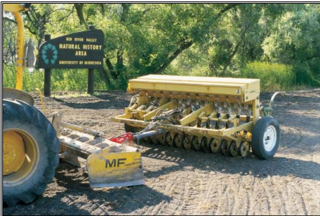
Figure 1.2: A specialised Truax drill planter, developed to also plant chuffy grass seed.
