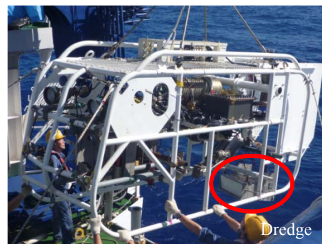
Fig.1 Picture of the Deep Tow and the dredge hanging its releaser.
