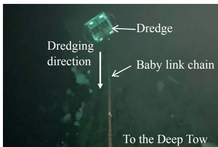
Fig.3 Picture of the dredge on the seabed
