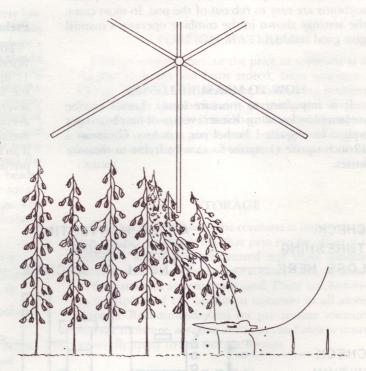
Reel position in relation to the cutterbar is an important consideration in minimizing losses. Set the vertical position of the reel so that it runs just deep enough to control the stalks. Deeper running causes more shattering. A pickup reel is helpful when beans are lodged.
