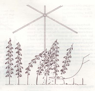
If the reel runs slower than the combine ground speed, it drags the stalks causing shattering.
