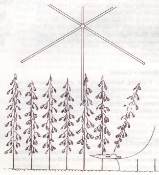
Excessive reel speeds cause stalks to fan and shattering results.
