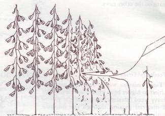
Fast ground speed in relation to knife cutting speed causes bean stalks to be pushed over and the knife slides up the stalk, stripping and shattering beans and pods. As plants are pushed over, they rub against each other causing a threshing process between plants. A combine speed of 3 miles per hour is an optimum speed in most soybeans.
