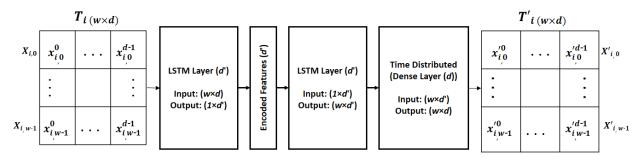
Figure 2.8: An LSTM-Autoencoder Network
