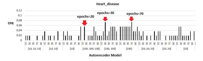
Figure 4.12: Stopping Points for Different Autoencoder Models for Heart\_disease Dataset
