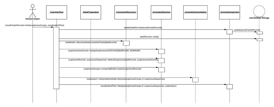
Figure 3.7: Sequence Diagram for Domain Expert Interaction Involving Anomaly Inspection
