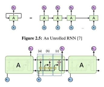
Figure 2.6: LSTM Structure [7]
