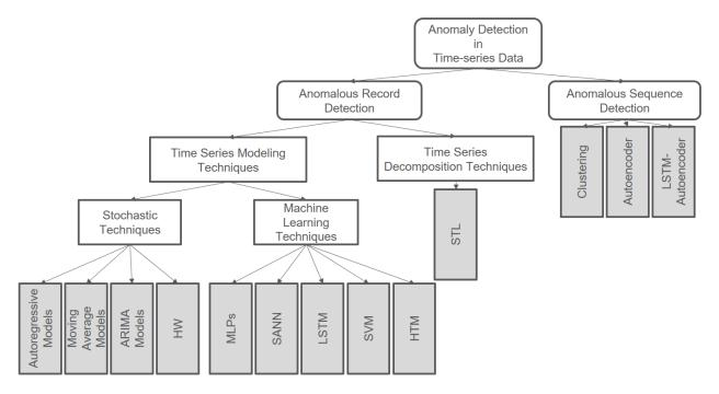
Figure 2.4: Classification Framework for Anomaly Detection Approaches for Sequence Data
