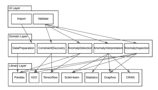
Figure 3.3: Logical View of ADQuaTe Tool Architecture
