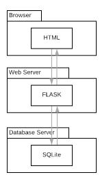
Figure 3.4: Deployment View of ADQuaTe Tool Architecture
