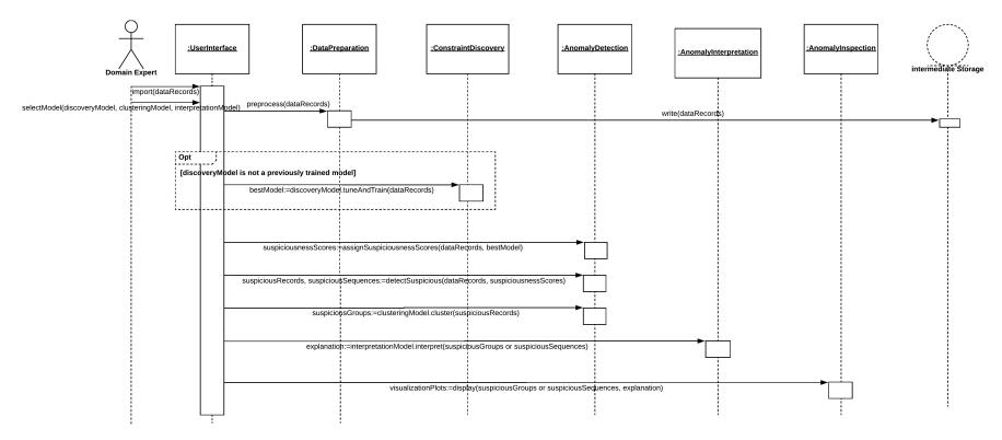
Figure 3.6: Sequence Diagram for Domain Expert Interaction Involving Data Importation
