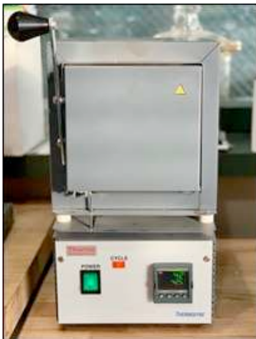
Figure 25: FB1315M Thermo Scientific Thermolyne furnace used to bake samples
