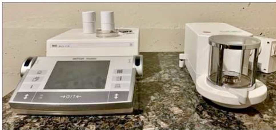
Figure 26: Mettler Toledo MX5 scale, with a readability of 0.001 mg
