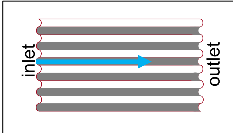
Figure 23: Linear analysis schematic, performed with XPS to obtain poison atomic percent distribution from inlet to outlet
