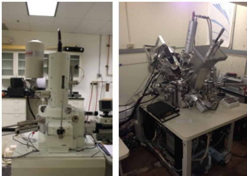
Figure 20: Used scanning electron microscope on the left, and X-ray spectroscope on the right [16].
