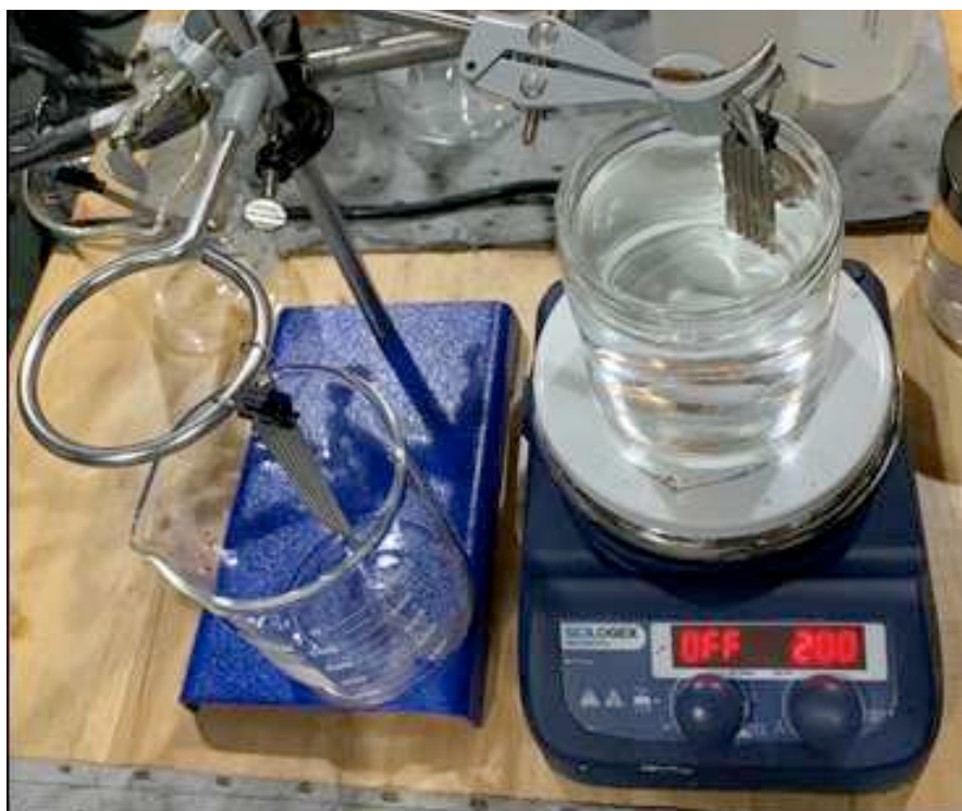
Figure 31: Scilogex hot-plate stirrer and washing setup
