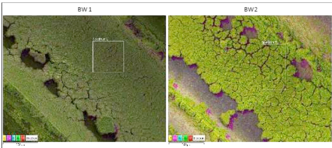
Figure 52: EDS layered image of middle samples baked first and then washed (BW1) and washed first and then baked (BW2)
