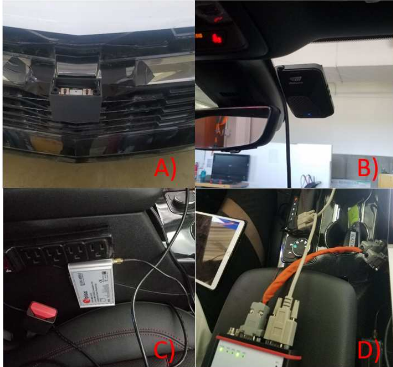
Figure 3.5: Physical locations of sensors on probe vehicle A) Radar mounted on front and center of vehicle grille B) Camera mounted on windshield slightly offset to the left C) GNSS Receiver mounted on center console, near-as-possible to vehicle center of mass D) Vector CAN interface mounted on center console
