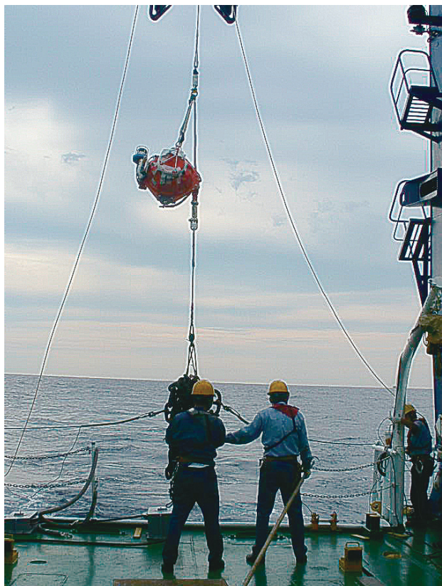
Fig. 10 Photograph of the acoustic transponder and the ceramic pressure-tight sphere being hung from KAIREI
