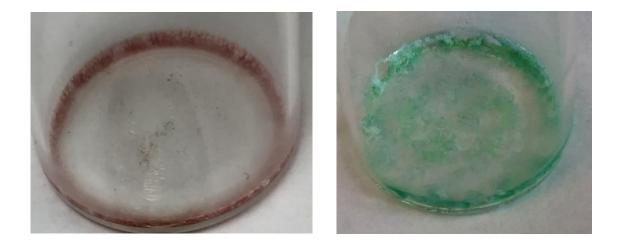
Figure 4.2. Photographs of crystals of  $Co(H_2O)_6(B_{12}F_{12})$  (left) and  $Ni(H_2O)_6(B_{12}F_{12})$  (right).
