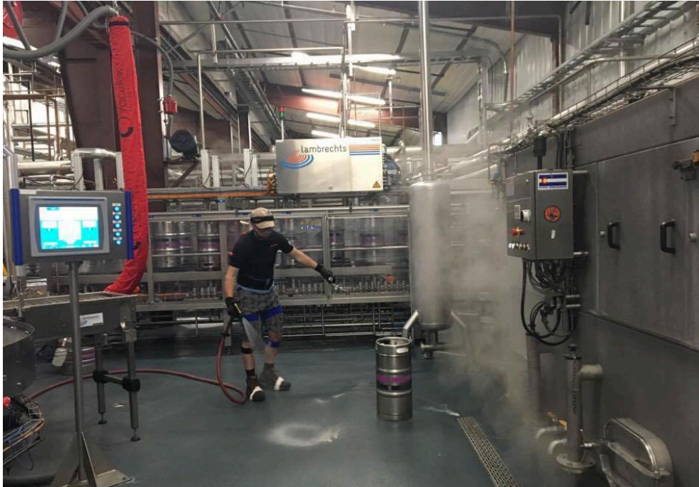
Figure 5.3. A worker cleans a floor with pressurized water next to a machine that cleans kegs
