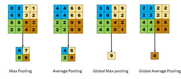
Figure 3.4: Various pooling techniques applied on a  $4 \times 4$ , two-dimensional data, with a pooling filter of dimension  $2 \times 2$ .
