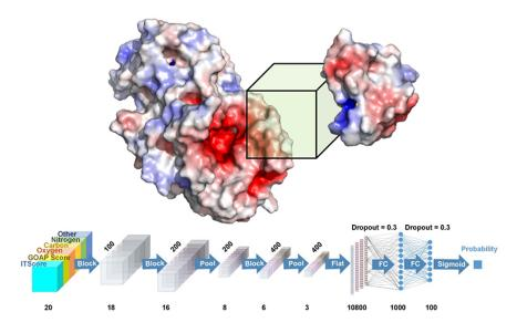
Figure 4.2: 3D CNN model architecture for DOVE. Picture used by permission
