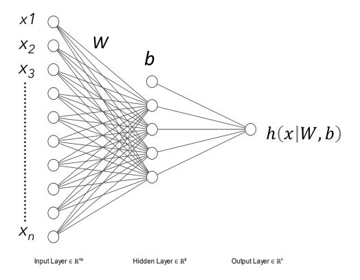
**Figure 3.1:** Feed-forward network with a single hidden layer. This image is generated using NN-SVG online tool [12]
