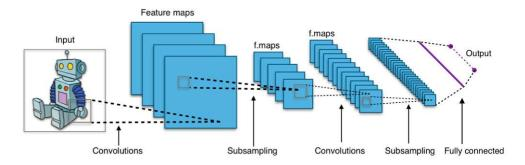
**Figure 3.5:** A depiction of 2D convolution on the images. The features extracted from the original image are down-sampled by applying pooling layers of different sizes. [15]
