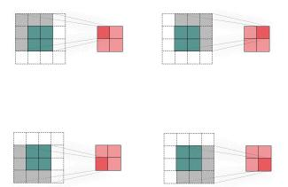
**Figure 3.3:** A  $5 \times 5$ , two-dimensional data, with a kernel of dimension  $3 \times 3$ , stride 1, and padding of size 1 [14].
