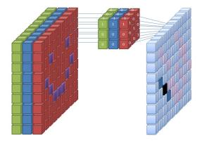
**Figure 3.2:** Features of a Convolution Neural Network consisting of multiple channels. The convolution operation is applied to a patch of the input data over all the channels for every iteration [13].
