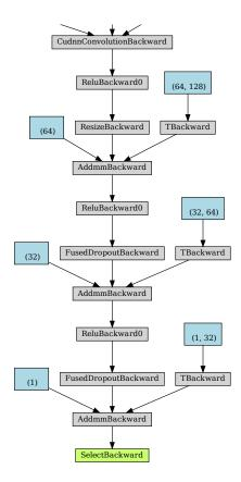
Figure A.2: The final convolutional block is connected to a block consisting of three fully connected layers
