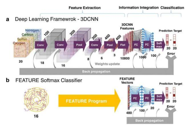
Figure 4.4: Deep 3D Convolutional Neural Network and FEATURE-Softmax Classifier models [18]. Picture used by permission
