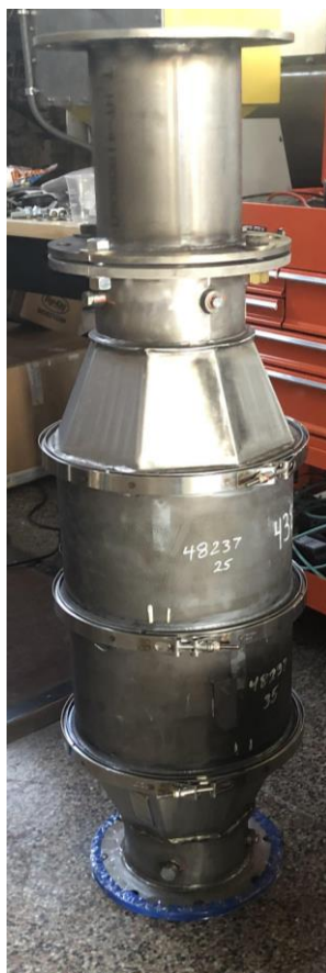
Figure 13: The two catalyst bricks are clamped together and then bolted into the exhaust using a series of adapters.
