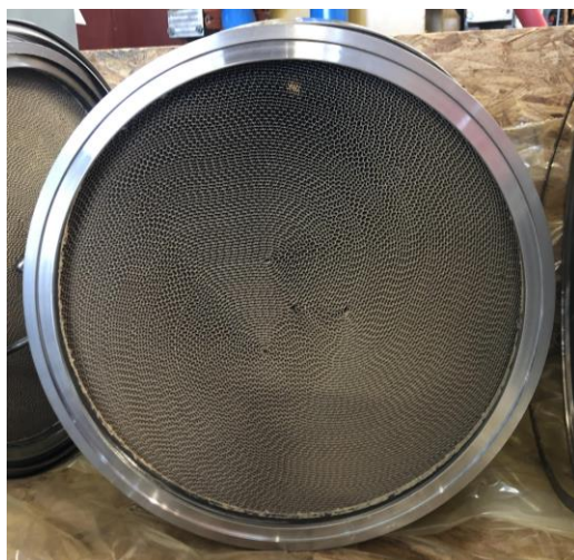
Figure 12: Cross sectional view of a catalyst brick. Two bricks are used in the standard configuration.
