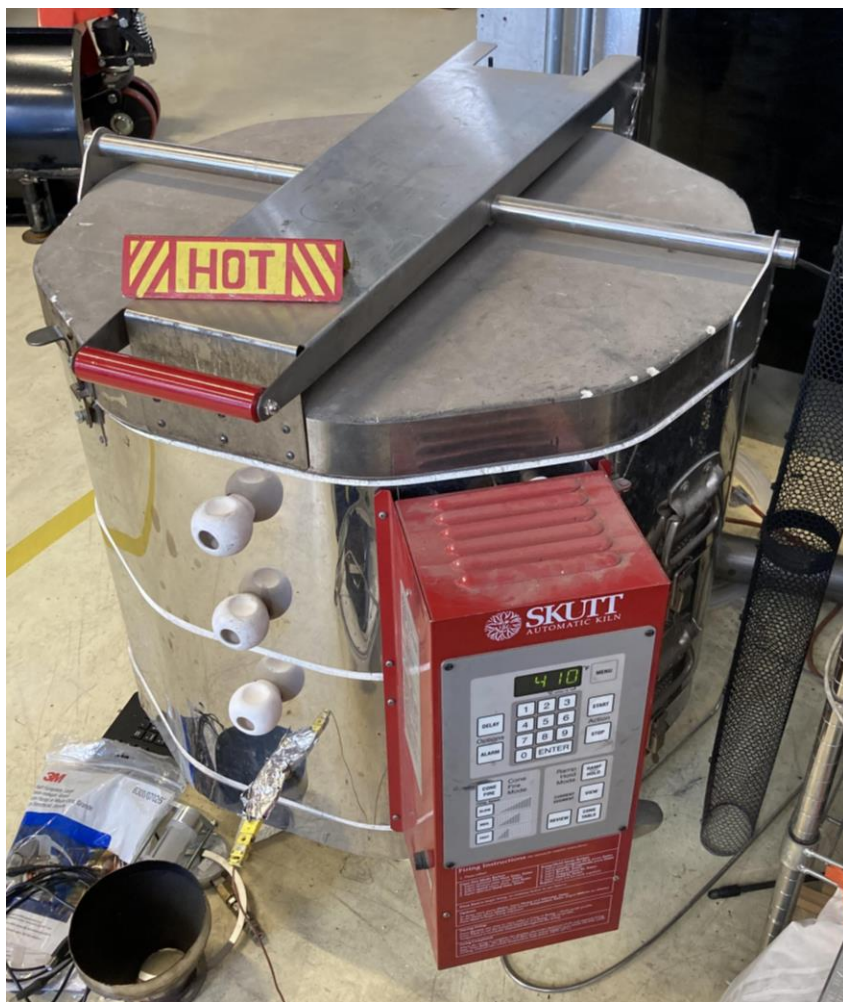
Figure 11: This Scutt automatic kiln was used for catalyst de-greening and aging.
