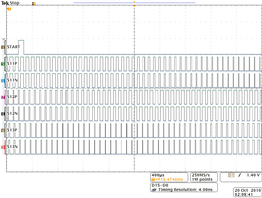
Fig. 58. Switching signals for output phase 1
