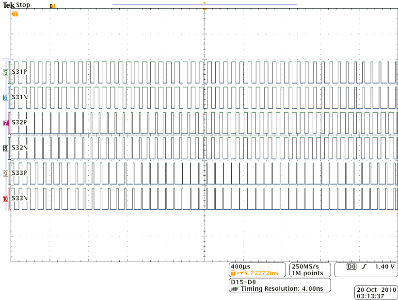
Fig. 60. Switching signals for output phase 3
