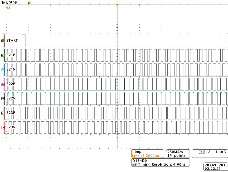
Fig. 59. Switching signals for output phase 2
