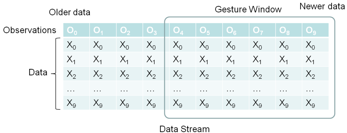
Figure 9: Example of a sliding window segmentation approach. In this example, the window size is 6, so the 6 most recent observations are used for recognition.
