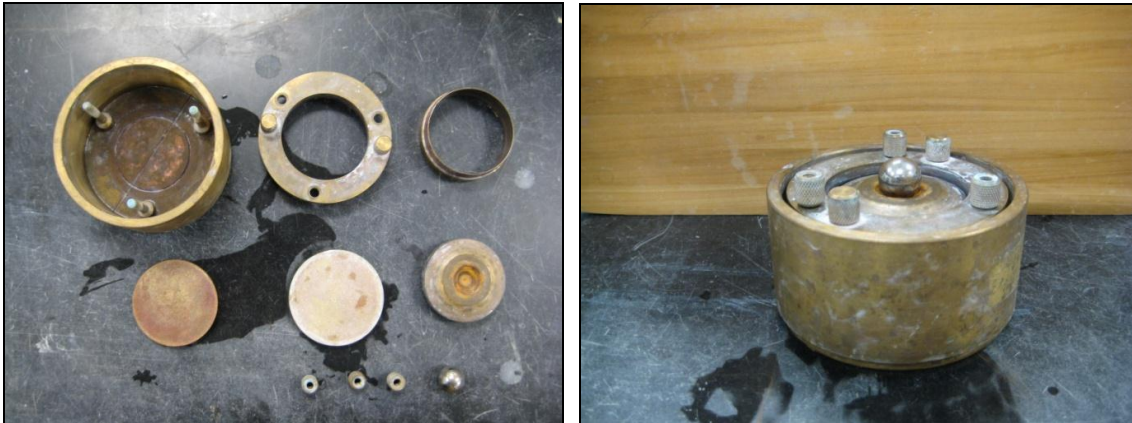
Figure 3-7: Shows consolidation tools like the ring, porous stones put separately and assembled.
