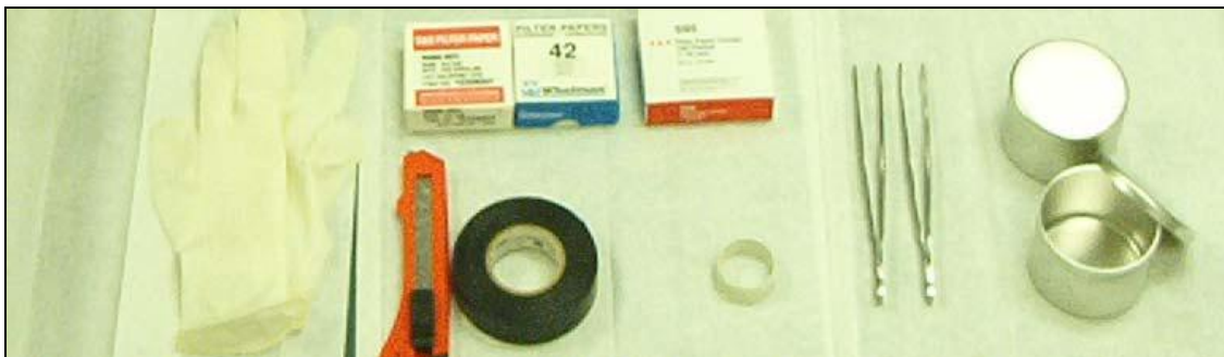
Figure 3-10: Filter paper, tins, tweezers, latex gloves, PVC ring, and electrical tape are shown in the picture. [Report No:TX-05/0-4518-1]
