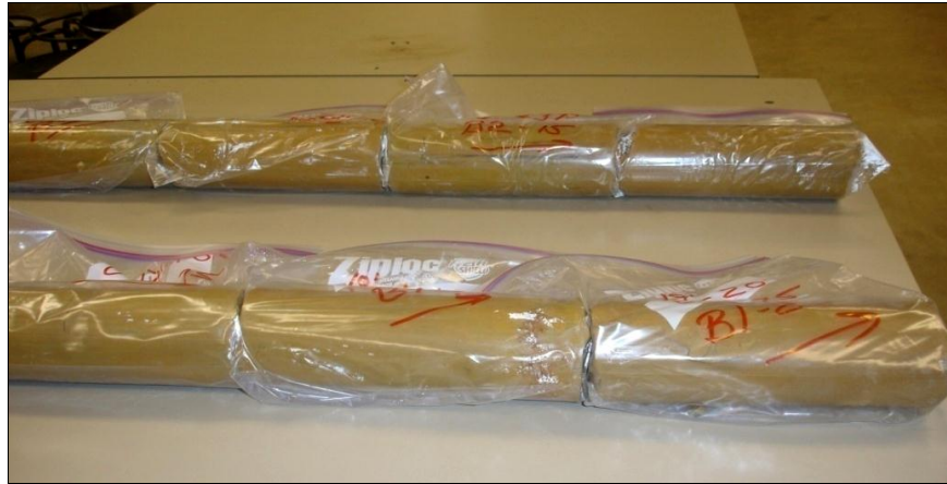
Figure 3-3: Extracted and wrapped soil sample from boreholes
