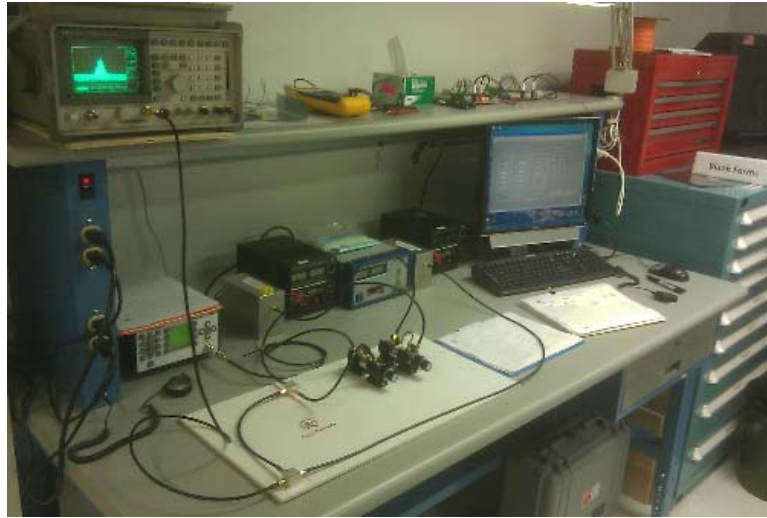
Fig. 14 Packet Loss Rate (PLR) testing arrangement implementation.
