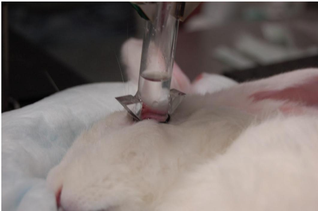
Figure 24. Photograph of the eye coupling device. Note that the double periscope configuration allows for a direct light path through the eye which, otherwise, would be blocked by rabbit's facial features.
