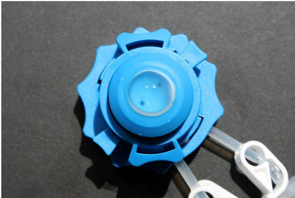
Figure 23. Photograph of an isolated cornea clamped on the artificial anterior chamber. Note that the clamping region is within the sclera which can minimize stress on cornea.
