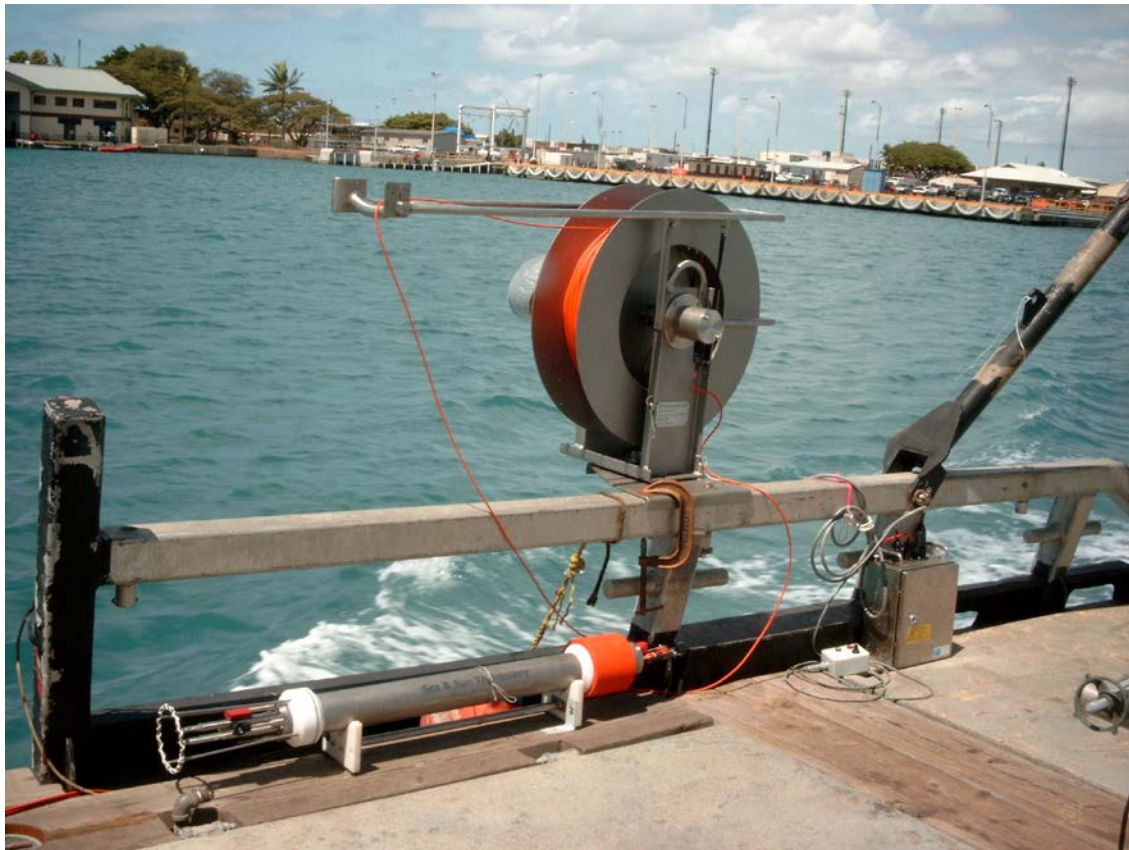
Figure 9. MSS-90 profiler and SWM2000 operational winch system during RASP measurement campaign.
