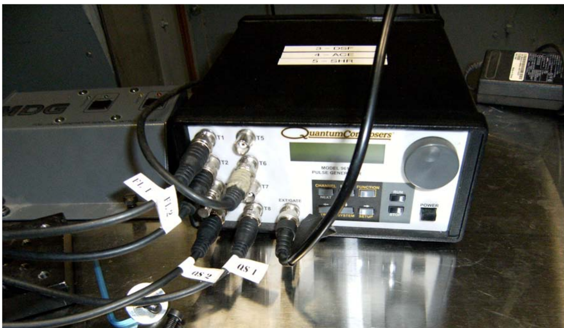
Figure 26. Quantum Composer connected to laser, camera, and motion controller
