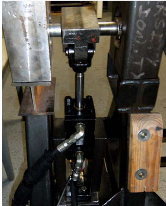
Figure 5. Linearly actuating hydraulic cylinder
