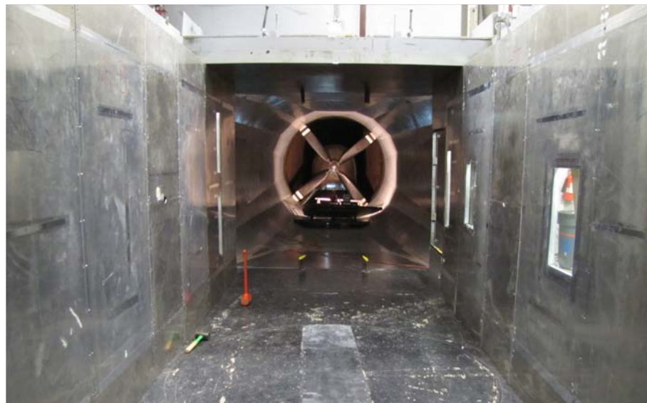
Figure 2. Reduced LSWT test section (7 ft \times 7 ft) – looking downstream
