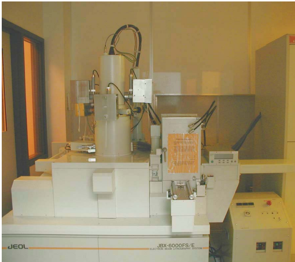
Fig. 68. E-gun chamber in room 1 (with load lock)
