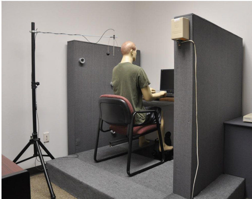
Figure 4.29. The manikin that was used as the human figure during airflow measurements.
