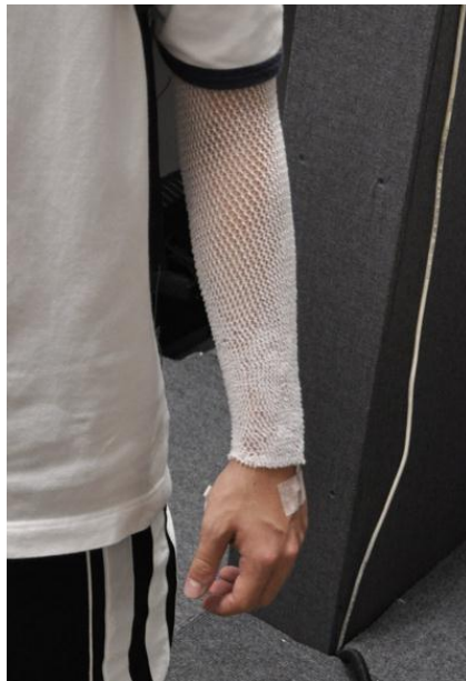
Figure 4.6. Medical mesh to secure thermocouples.
