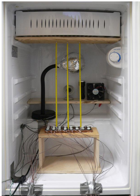
Figure 4.21. Modified refrigerator that was used as calibration chamber.
