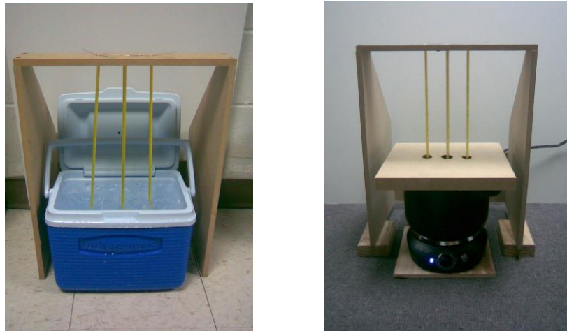
Figure 4.19. Images from the actual ice bath and the boiling point calibration setups.
