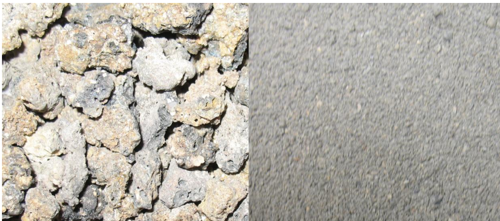
Fig. 18. Agglomerated ash by slagging and the normal ash.
