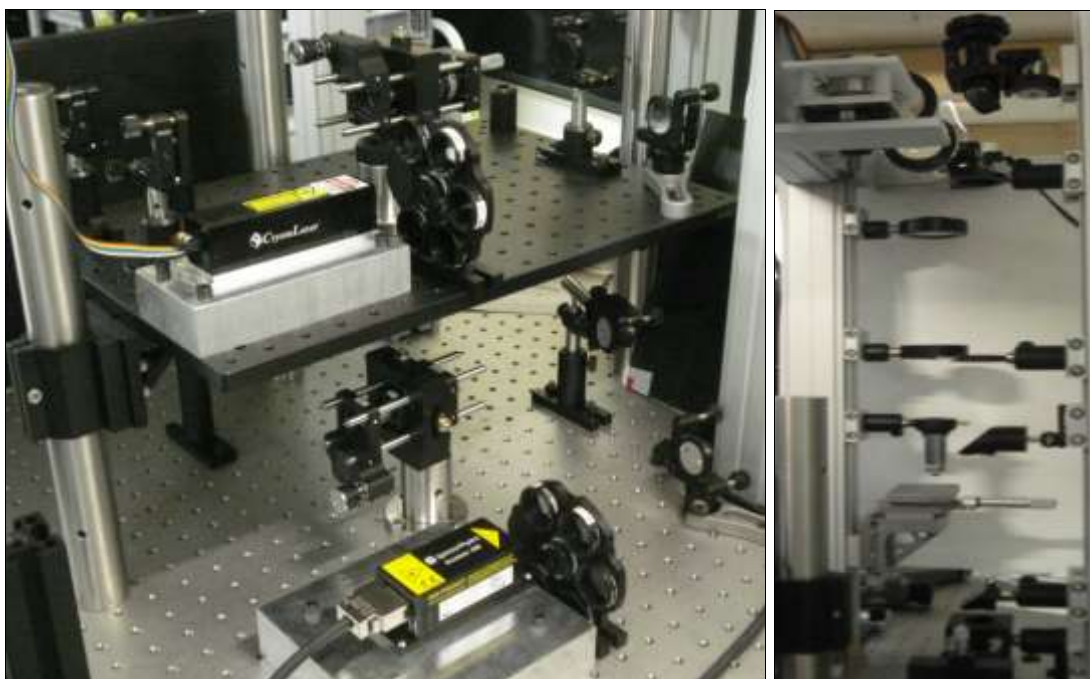
Fig. 7. Images of the constructed bench top confocal reflectance and fluorescence microscope.
