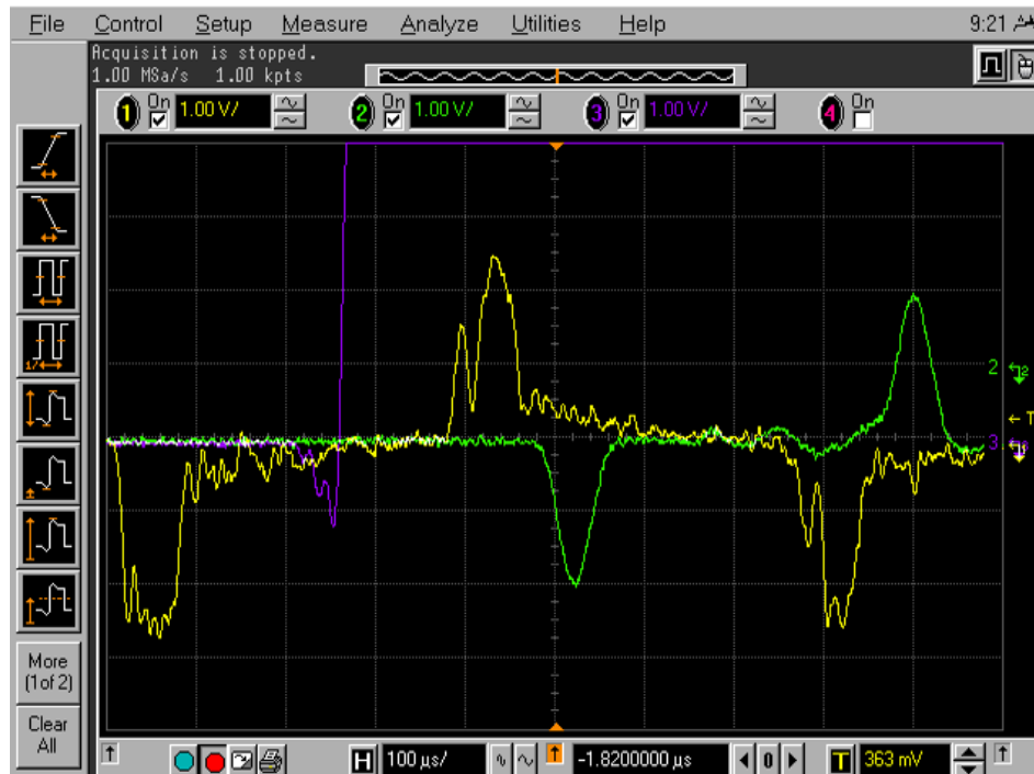
Fig. 10. Sample of wave signal output from strain gauges attached to SHPB set-up
