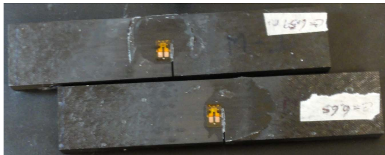
Fig. 9. Picture showing position of strain gauge bonded very near to crack-tip
