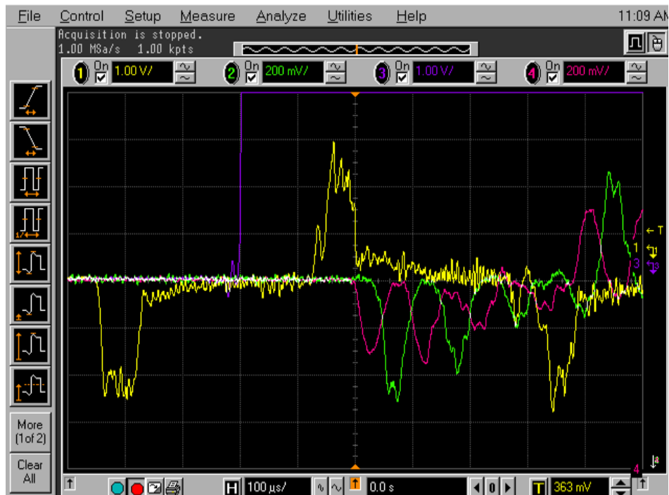
Fig. 18. Strain gauge signals recorded for Mode-II impact tests
