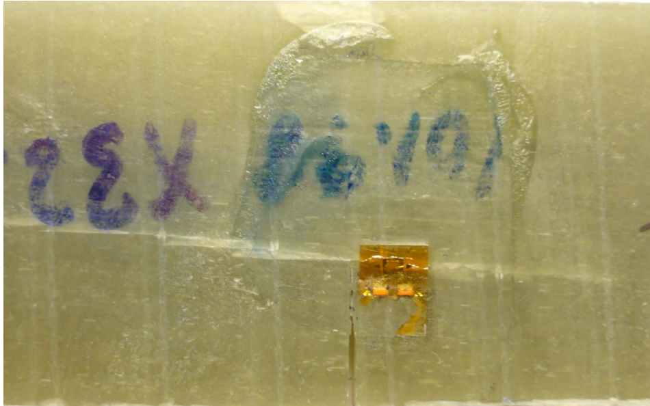
Fig. 17. Impact damaged fiberglass-epoxy laminate
