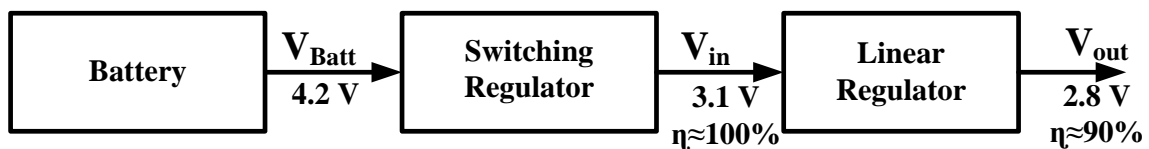
Fig. 1.2. Increasing Power Efficiency of LDO
