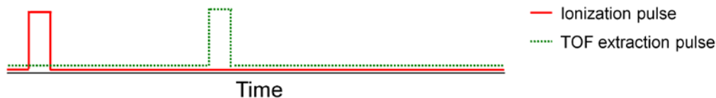
Figure 7. A schematic diagram of a single-stage time-of-flight extraction source showing both continuous extraction mode (a) and a pulsed extraction mode (b) taking advantage of time-lag focusing , also known as delayed extraction .
