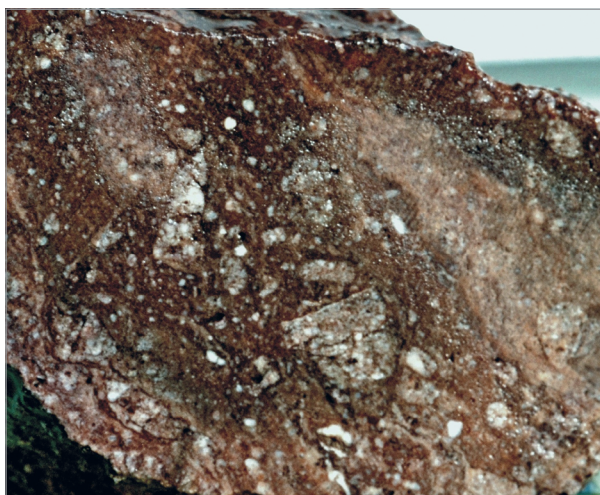
Figure 10. Polymict lithic impact breccia intensely silicified with clastic texture and aspect of fluidal texture. A sample from this exposure at the top of the central uplift, an intensely silicified sample of which gave thin sections that displayed planar deformation features (PDFs) in quartz clasts (SM348; see Fig. 16b).
