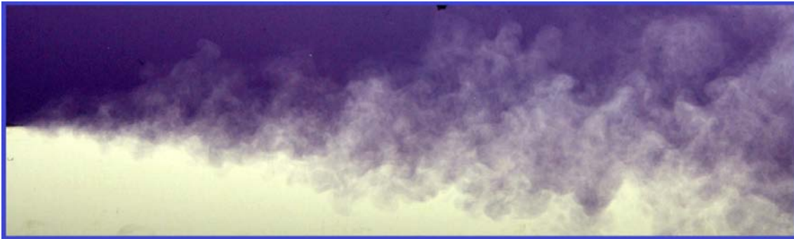
Figure 20: Dye visualization of RTI.
