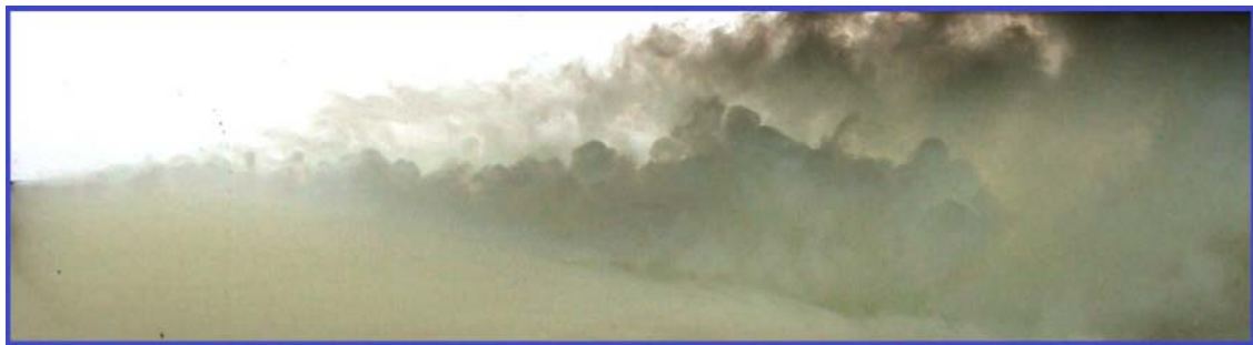
Figure 19: Milk visualization of RTI.
