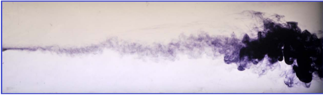
Figure 21: Dye streaklines from flapper tip.
