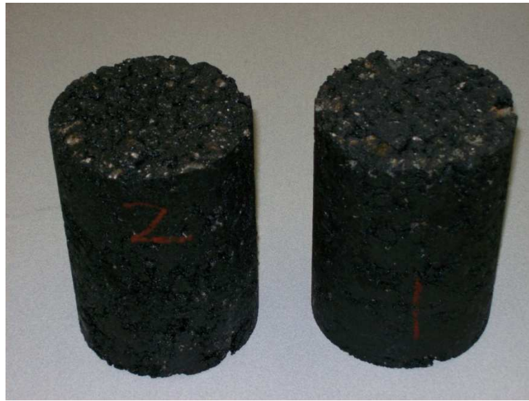
Figure 18 Superpave Gyratory 4 Inch Diameter Specimens
