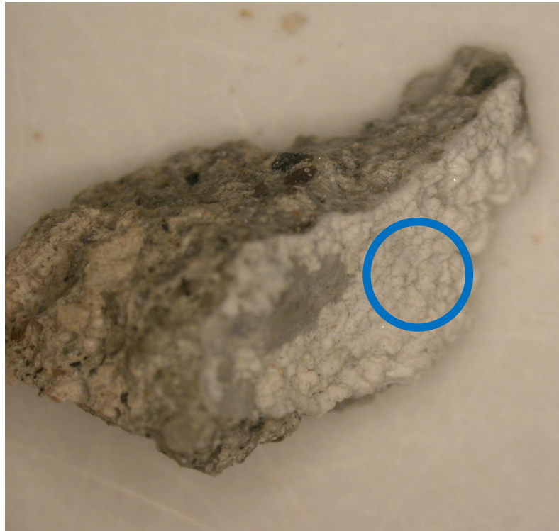
Figure 6 Stereomicroscope Image of Gel on Surface of ED RCA Particle at TTI
