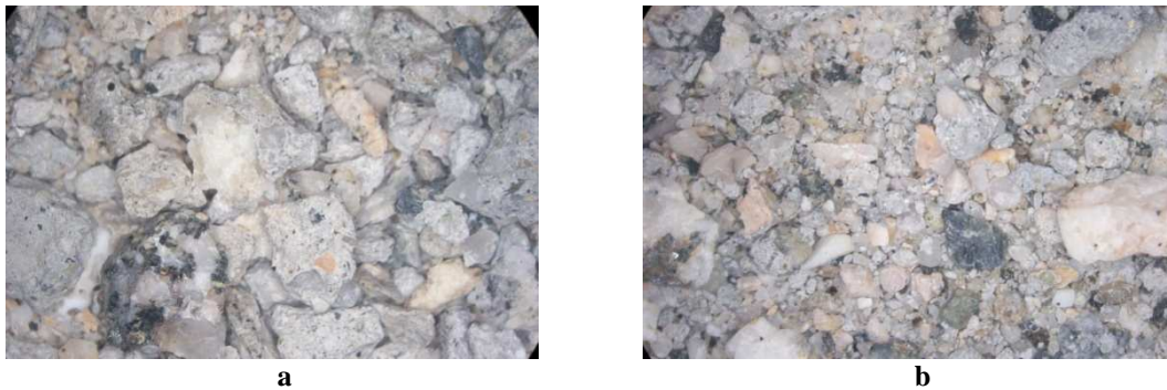
Figure 85 Stereomicroscope Images of Fine ED RCA Particles (a) Before and (b) After Micro-Deval Testing
