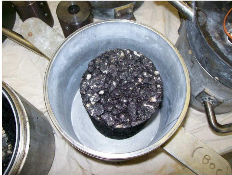
Figure 19 Superpave Gyratory Specimen in Dilatometer
