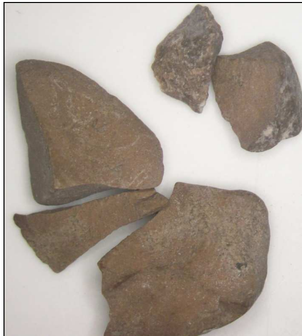
Figure 86 Stereomicroscope Image of Shattered Limestone Aggregate from HL RCA Coarse Aggregate Freeze-Thaw Test
