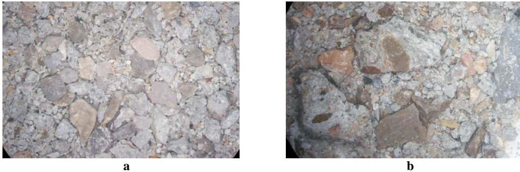
Figure 84 Stereomicroscope Images of Fine HL RCA Particles (a) Before and (b) After Micro-Deval Testing
