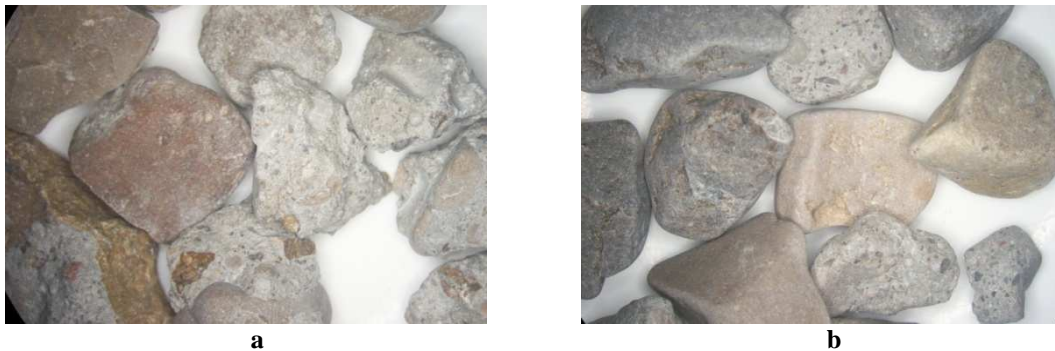
Figure 83 Stereomicroscope Images of Coarse HL RCA Particles (a) Before and (b) After Micro-Deval Testing
