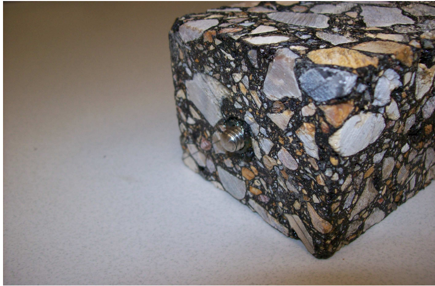
Figure 20 Measuring Stud Mounted in the End of Sample Beam
