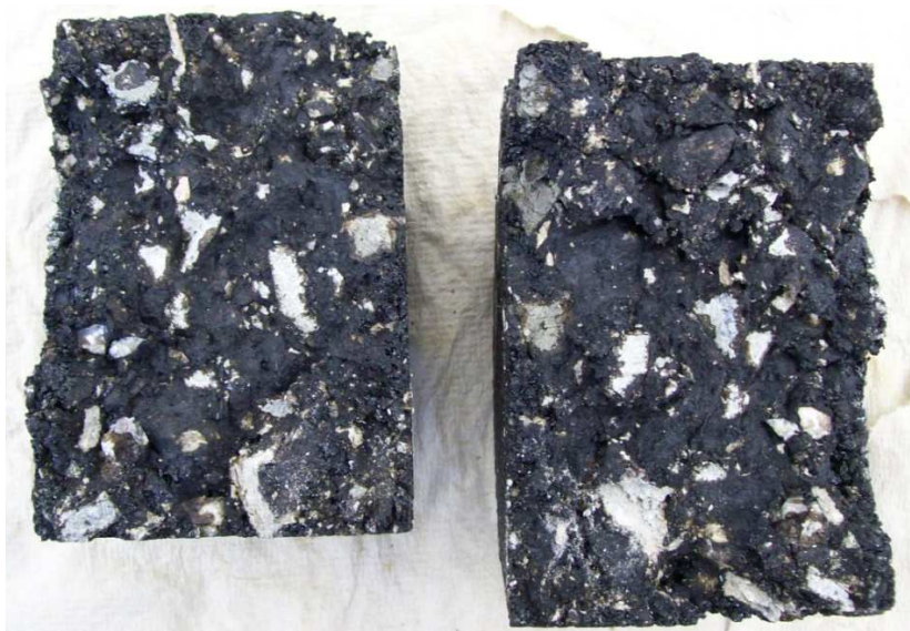
Figure 75 Fracture Cross-Section of ED RCA Specimen Conditioned in Water for 24 Hours
