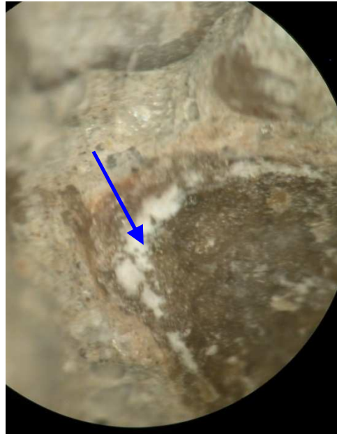
Figure 12 White Material and Aggregate Rim on Holloman Sample 6, Stereomicroscope
