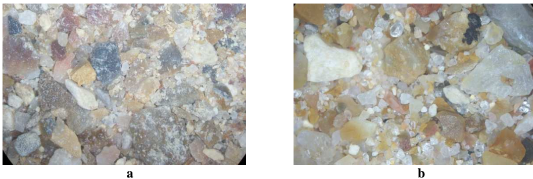
Figure 82 Stereomicroscope Images of Chert Particles (a) Before and (b) After Testing in the Micro-Deval
