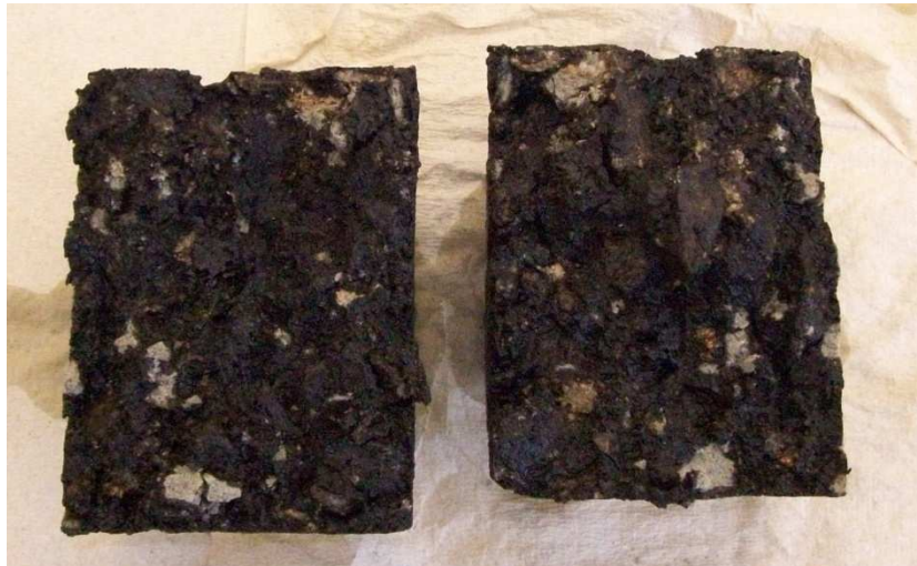
Figure 76 Fracture Cross-Section of ED RCA Specimen Conditioned in Water for 6.5 Days
